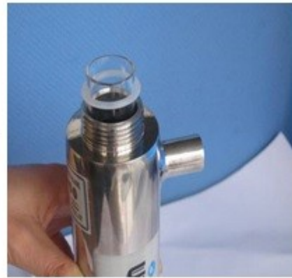
2. Put the O-ring on the quartz sleeve
